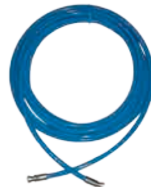
Ref. 18510 Antipulsation hose Ø 3/8" with M16x1,5 fitting, 15m
