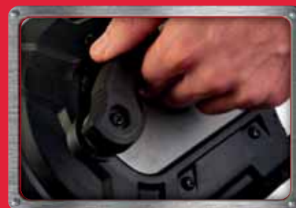
Tool-free blade locking mechanism
