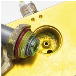
Sealant contamination in the A/C service unit without the use of the Recycle Guard
