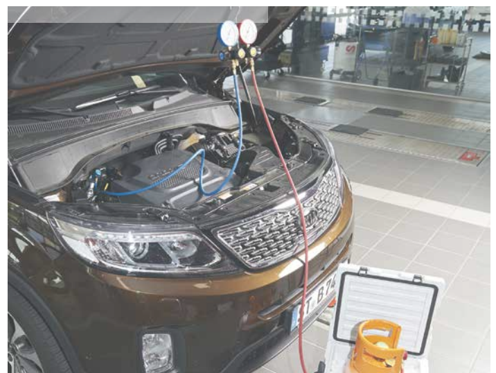
During the condensation process the pressure is monitored by a 4-way manifold
