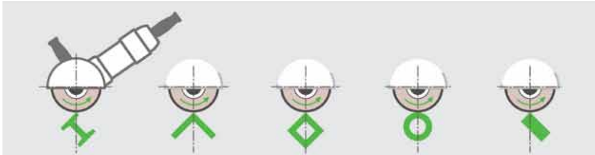
Proper cutting methods of various metal forms.
