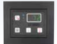
The Passport Compact keypad/display features a simple three-button layout and built-in bezel
