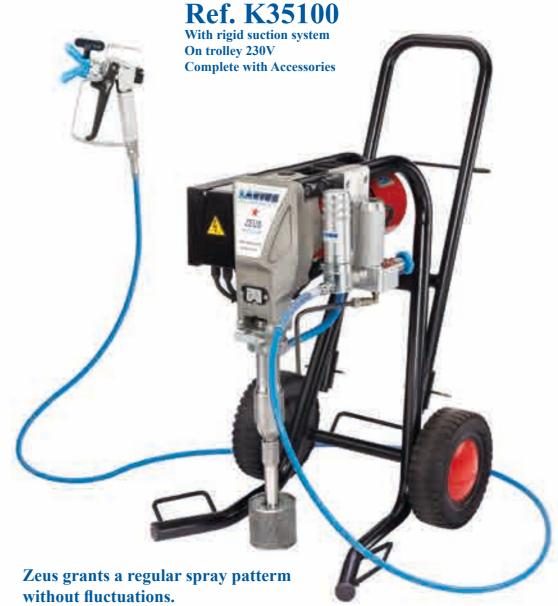
**Technical Data** Max delivery 4 l/m **Motor power** 2,0 Kw Max. pressure 220 bar 230 VAC - 50 Hz Voltage 115 VAC - 60 Hz Weight on trolley 58 Kg 1 Gun 0.029" Max. nozzle size 2 Guns 0,017"
