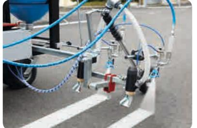
Technical features Motor power 10 HP by Yamaha 230 bar Max. pressure Max. flow rate 4,5 l/m **Dimensions** 1650x750x1000 Weight 220 kg Multi-purpose:
