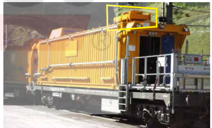
Radiator mounted separately on wagon roof
