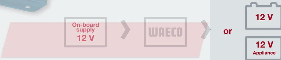
**The IU charging converter is simply integrated into the wiring of the starter and leisure batteries. Raising the charging voltage to 14.2 volts, it ensures optimal charging during the drive.**
