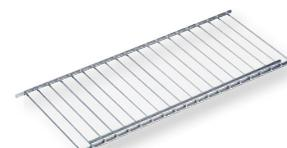
**Ventilation grill for single and double-door models:** Attached to the outside of the vehicle. single-door models require the grills LS 100 (top) and LS 200 (bottom). The LS 300 for RML and double-door models can be used at the top and at the bottom.
