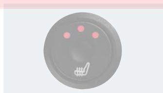
Level 3 = High heat output for fast heat-up when you set off
