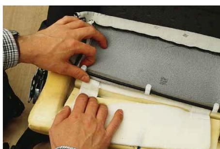
Simple installation: just insert the heating elements between the foam core and the cover
