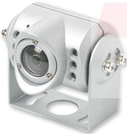
The lens is shielded by a replaceable stone chip protection screen. The use of a shutter was deliberately omitted to prevent the risk of scratching by trapped dust particles.
